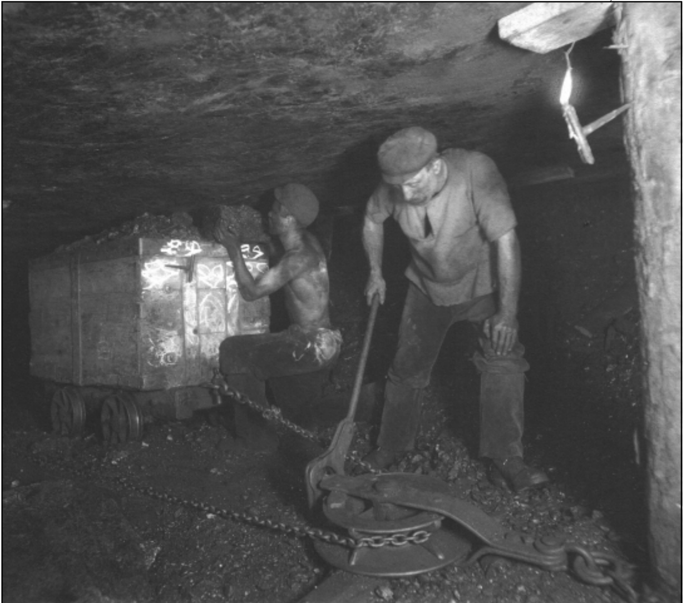
Frog Lane Colliers loading coal into Drams at the Coalface - Courtesy of Ann Matson
